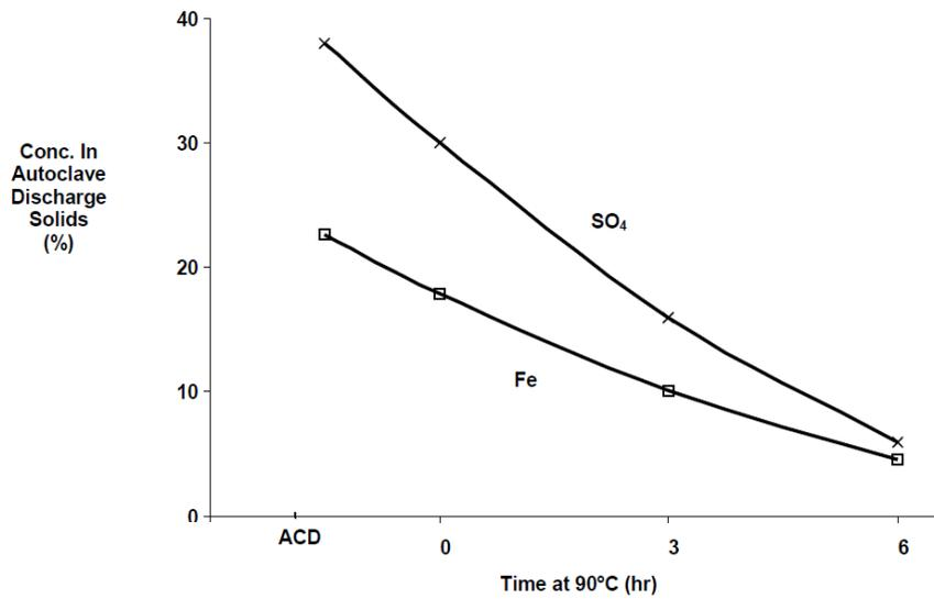
Figure 3 Concentrations of iron and sulphate in the solid residue discharge from autoclaving Quimsacocha flotation concentrate as a function of hot curing time
