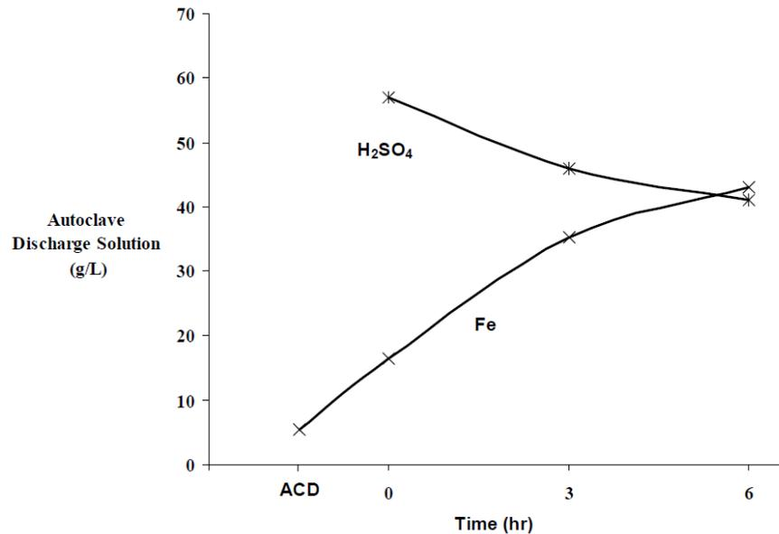
Figure 4 Concentrations of iron and sulphuric acid in solution in the discharge from autoclaving Quimsacocha flotation concentrate, as a function of hot curing time.
