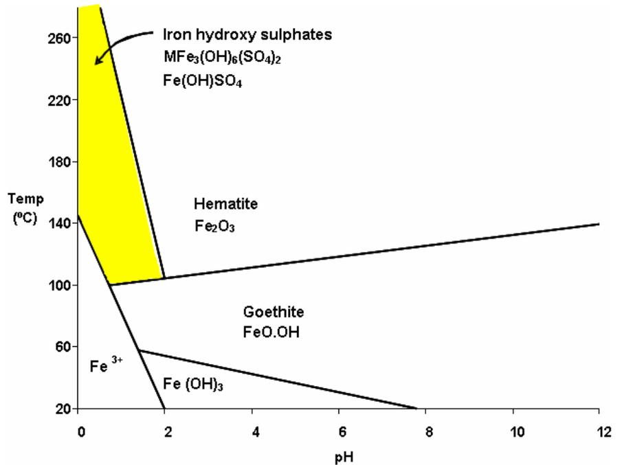
Figure 1 Areas of stability of various compounds in the Fe-S-O system (After Babcan [2])
