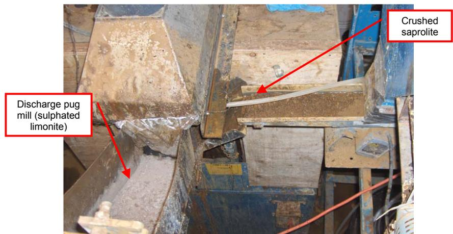
Figure 7 Photograph of Ball Mill Feed Trough
