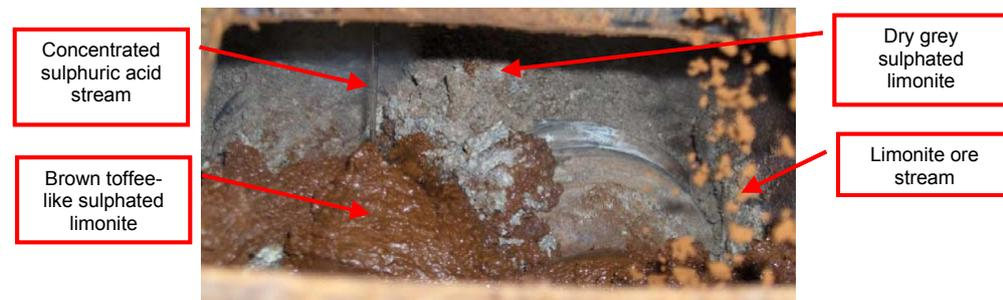
Figure 6 Photograph of Formation of Sulphated Limonite
