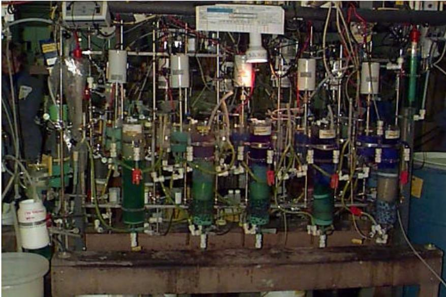
Figure 18: Ni/Co SX Circuit View
