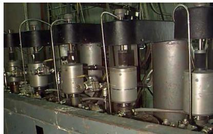
Figure 3: Continuous Autoclave Agitator Assemblies
